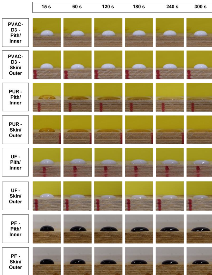
Figure 6. Droplets of the different commercial glues showing contact angles on the surface of the bamboo adherend at different time intervals.
